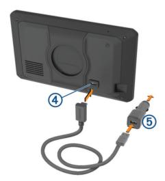
4 Plug the other end of the vehicle power cable into the vehicle power adapter 5.
